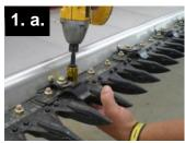
a. Starting 12"/30cm from the right side of the header and every 12"/30cm across the header, remove the guard nut and bolt from the guards.
