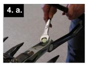
a. Using a 3/4"/19mm wrench, loosen the adjustment bolt.
